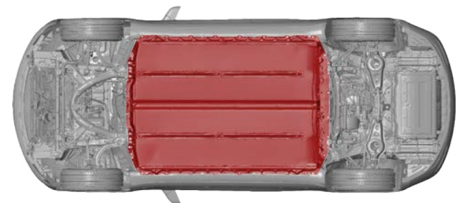
Native EV battery pack architecture (example)
