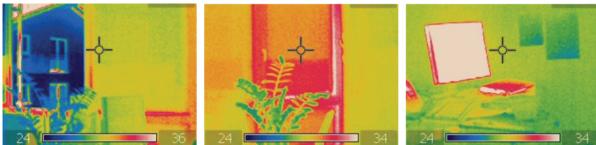
Figure 4: Inside view on façade with an open and closed windows (left), a up heated window from solar radiation (middle), both with no direct sunlight but summer outdoor conditions, in false colours for radiation temperature. View on inner wall with working place (screen and notebook) under equal conditions for comparison.
