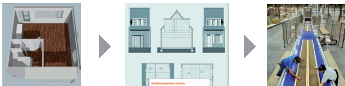
Figure 4 – 3D scanning, BIM generates technical drawings based on existing concepts, flexible factory makes prefab solutions (Source: Energiesprong, 2014)
