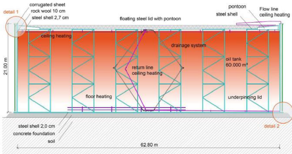
Figure 41. Reconversion solution for the existing tank of 60,000m 3 to be used as STES. Source: Solites.
