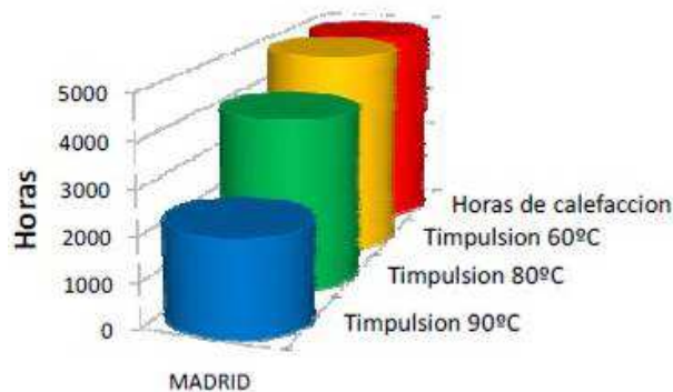
Hours with condensing possibilities for natural gas with different impulsion temperatures for heating Source: Enercom
