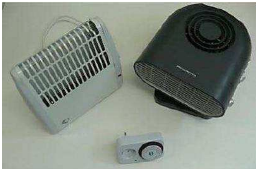
400 W (left) and 1200 W (right) radiators used for thermal excitation of indoor of dwellings, activated by programmable connectors (centre)
