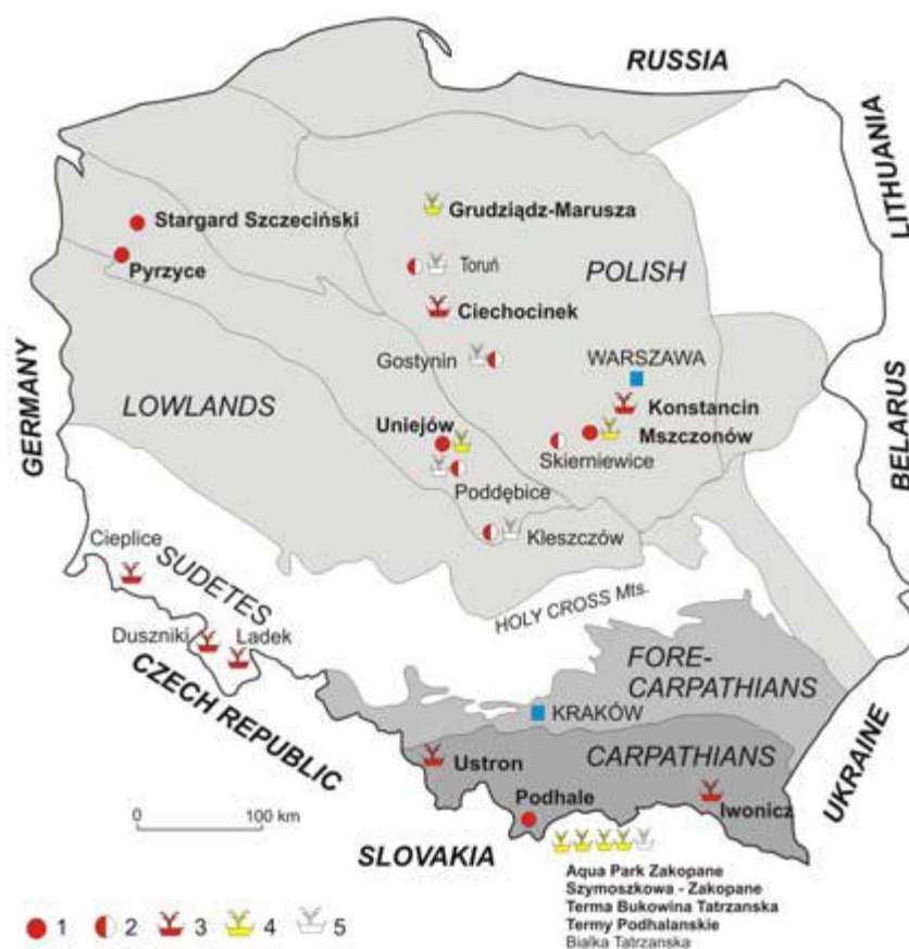
Fig. 5. Poland, 2009: 1. geothermal heating plants in operation, 2. geothermal heating plants in realization (wells drilled or in drilling), 3. spas using geothermal waters, 4. geothermal bathing centres opened in 2005 - 2009, 5. geothermal bathing centres under construction (wells drilled or in drilling). Division into geothermal provinces after Sokolowski (1993)
