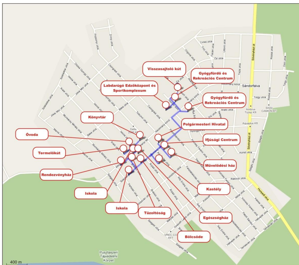
Fig. 7. The geothermal cascade system of Sándorfalva
