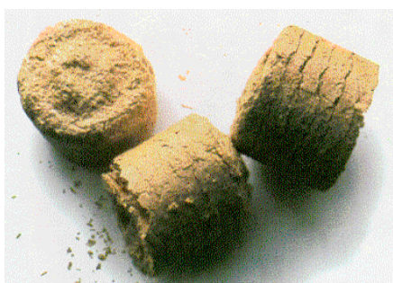
Fig. 3.7 Examples of wooden briquettes (left – diameter 50 to 75 mm, moisture content 5-20%) and wooden pellet (right – diameter , 8 and 12 mm, moisture content 6-10%).
