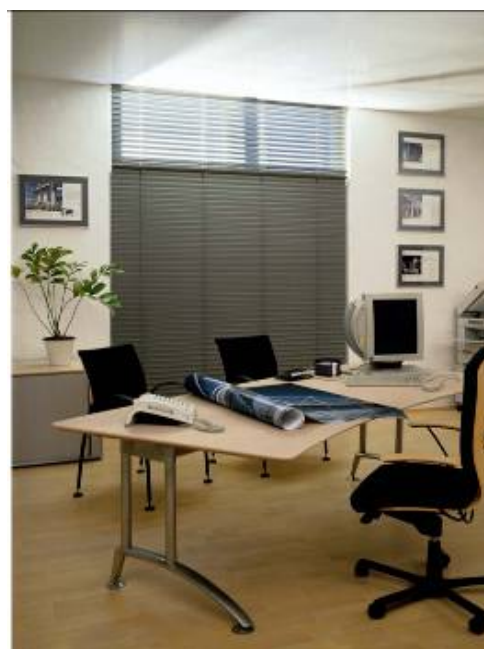
Fig. 2.3 Example of a Venetian blind with two parts that may be controlled individually: Solar shading in the lower part and daylight blinds in the upper part. (Photo: Vental).
