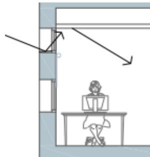
To guaranty good reflection factors, the reveal will be in aluminium. Depending on the upper surface finish (the finally selected product), the reflectivity may vary between 80% and 98%. The ceiling is covered with plaster.
