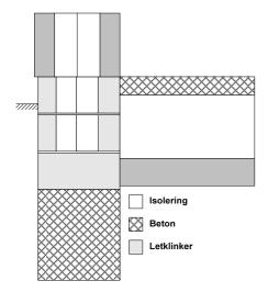
On this figure is shown a section of a joint between the outer wall/foundation/slab-on-ground. The insulation in the outer wall continues into the foundation.
