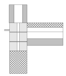
On this figure is shown a section of a joint between the outer wall/foundation/slab-on-ground with three insulated lightweight concrete blocks in the foundation.
