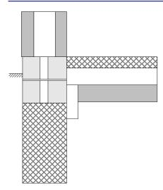
On this figure is shown a section of a joint between the outer wall/foundation/slab-on-ground with vertical insulation inside of the foundation.
