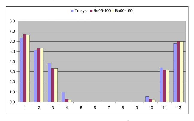
The yearly energy need for space heating has been calculated to 26,0 kWh/m² and 25,2 kWh/m² by the two programs, respectively TRNSYS and Be06, which means that the agreement is quite close.
