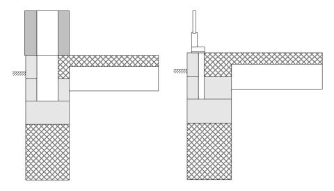
On these figures are shown sections of a joint between the outer wall/foundation/slab-on-ground respectively door/foundation/slab-on-ground. The insulation in the outer wall continues into the foundation.
