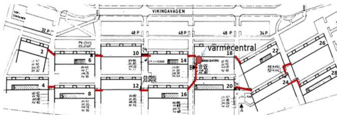
Figure 2.10: Shows the routing of the culvert network with the secondary circuits that LKF owns
