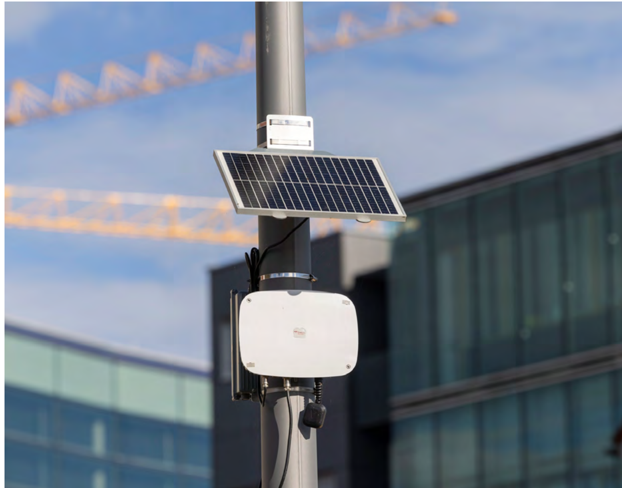
The IMAGINEXT project, co-funded by EIT Urban Mobility, is piloting an AI-driven Software as a Service solution to measure air quality in Lindau, Germany. Sensors installed in Lindau are assessing air quality changes before and after the reconstruction of cycling streets. ©EIT Urban Mobility
