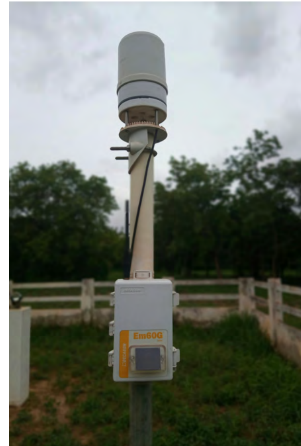
Weather station connected to a lamppost in Burkina ©Yoda Adaman, Unsplash
