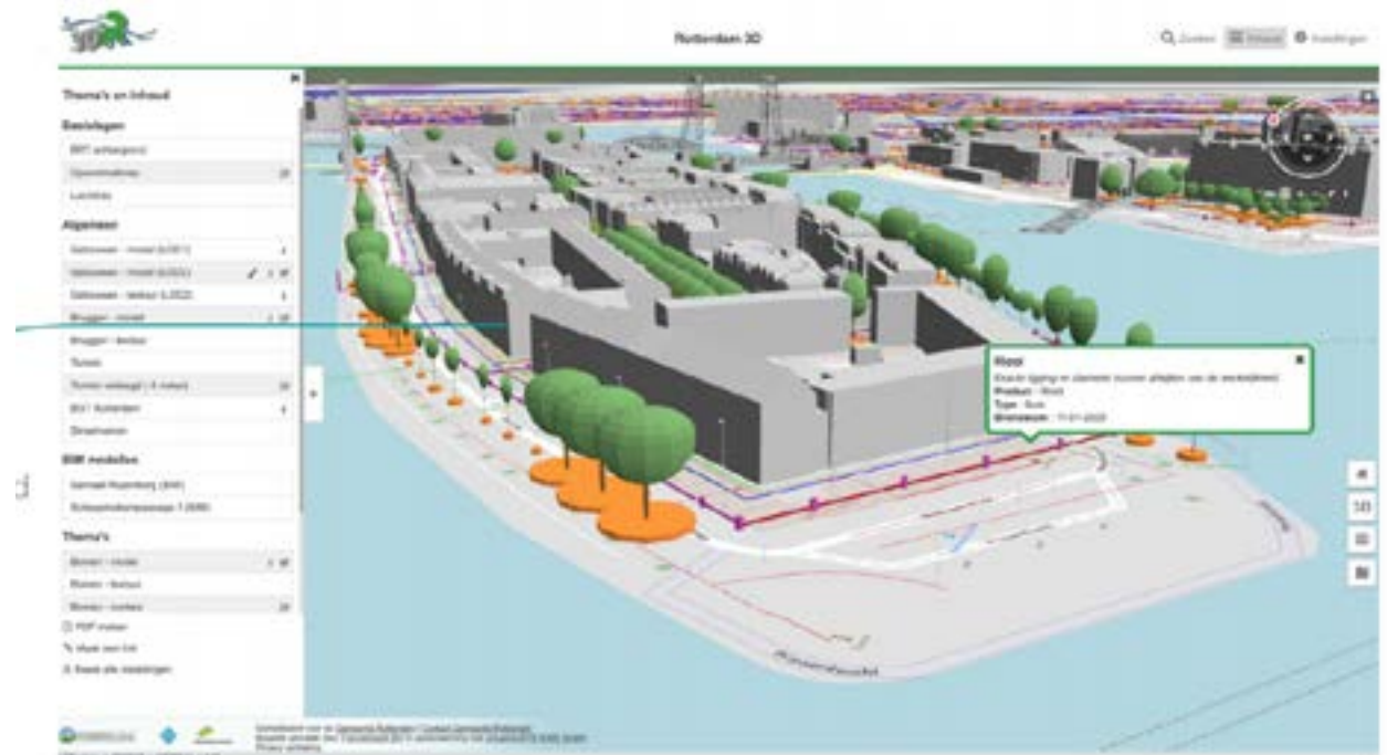
Figure 1 Two representation of the Digital Twin of Rotterdam: detailed buildings and attributes of objects above, and utility networks and other objects as trees below.
